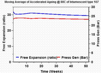
**TENMAT** Intumescent FF107 demonstrates stable behaviour over a simulated 40 year period with little degradation in properties and performance.
